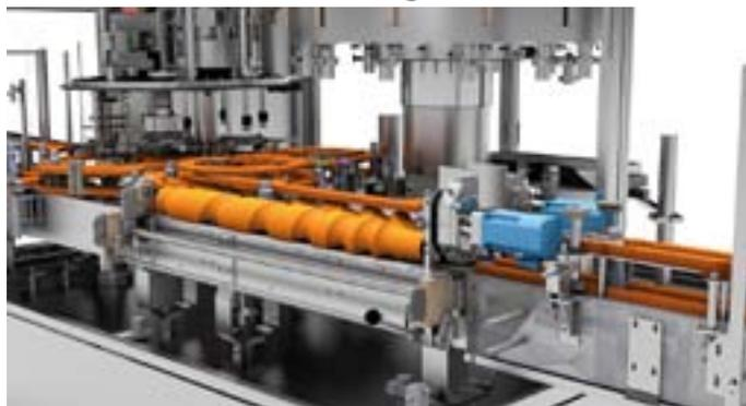
The machine still uses the weight-filling technology, known for its precision, reliability and cleanliness. Dosing cleanliness is further improved by using an analog probe which ensures real-time monitoring and filling of the tank in order to optimize the gravity flow.
