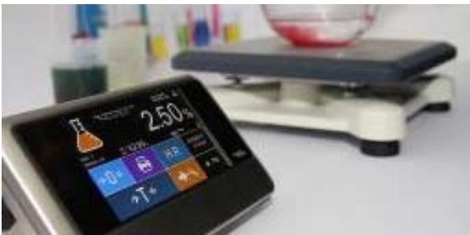
CSV files and to personalize your ticket. The R1TP weighing platform is light (less than 10 kg), movable and resistant. A new shock absorbing system includes patented stops which protect the sensor from potential overload.
