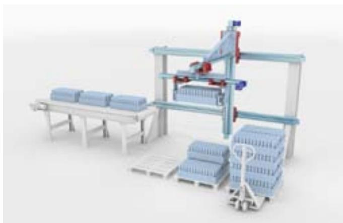
This linear axis is thus well adapted for the packaging industry where cardboard dust generally reduces the service life of linear guides.
